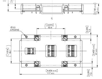
Note: Drawing shows adaptor to suit F203 triple output DC:DC Converter
